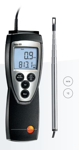
testo 425 is a compact anamometer with a fixed thermal flow velocity probe. The probe head has a diameter of 7.5 mm. With the extendable telescope (length max. 820 mm), the measuring instrument is suitable for flow velocity measurement in ducts. The testo 425 also measures extremely accurately in the low flow velocity range. The volume flow is directly shown in the display. For the purposes of volume flow calculation, the duct area can be
