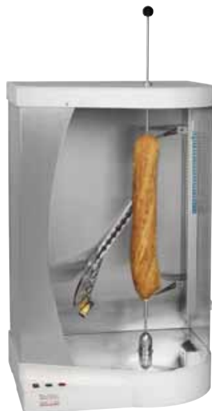
The laser sensor will move in a half circle around the sample.
