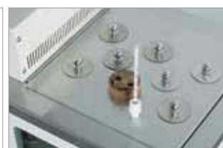
Easy holding of U-shaped viscometer glass tubes (optional)
