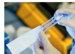
In the FibreBag method, digestion and filtration are carried out in a generously dimensioned filter bag made of a high-precision special textile that standardises reproducible filtration conditions. The FibreBags are incinerated together with the sample residue at the end of each digestion process. This single use means that each analysis is always conducted under the same standardised filtration conditions, thereby generating precisely reproducible results.
