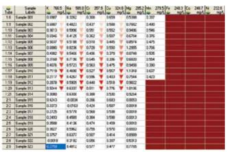
Using Fast Sequential AA, samples are only aspirated once and all elements are measured before progressing to the next sample.
