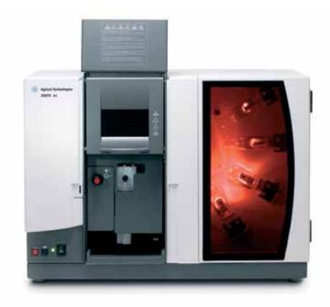
Conventional AA determines only one element at a time, so samples are analyzed time and time again during a multi-element sequence.
